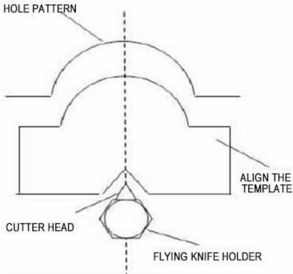
Figure 2 Schematic diagram of the centering of the hole processing tool head
